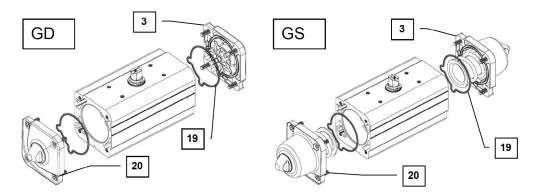
**Caution.** The Spring Return end caps cartridges (Parts N° 3 + 18+24+19+23+22+21) are a safety device, where the preloaded spring is set to avoid the dangerous spring jumping. Do not release the screw (part N° 21) to remove the spring from its seat, this operation must be done by ACTUATECH technician only.
